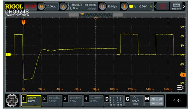
Fig. 7. Measurement: BEMF measurement cycle with optimized implementation
