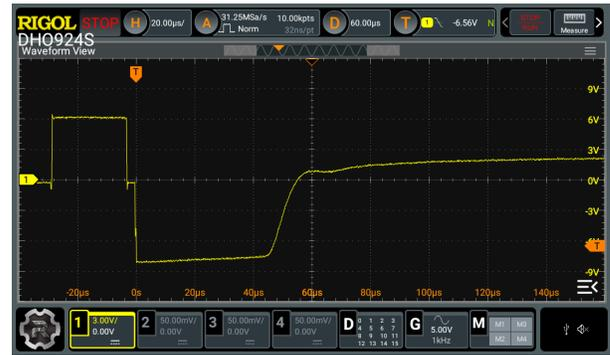
Fig. 4. Measurement: negative voltage spike at the start of BEMF
