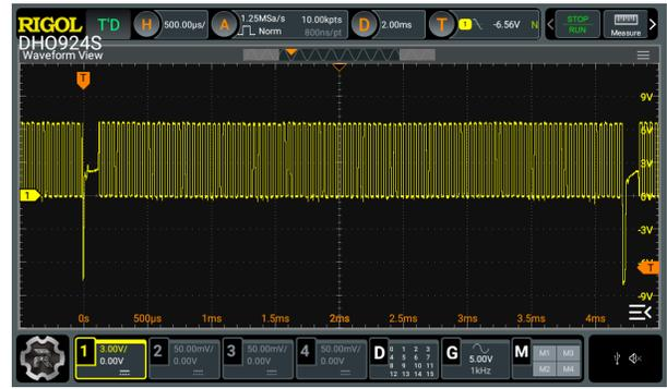
Fig. 6. Measurement: optimized implementation - motor voltage at 50% duty cycle
